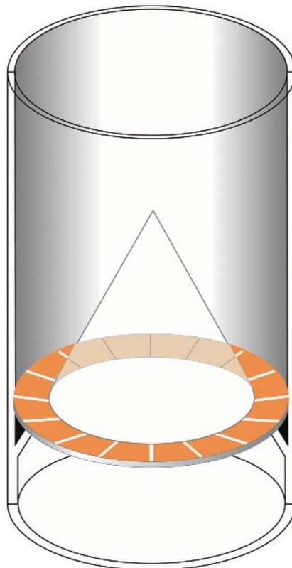
Figure 1. Silo with central cone for the cement industry.
